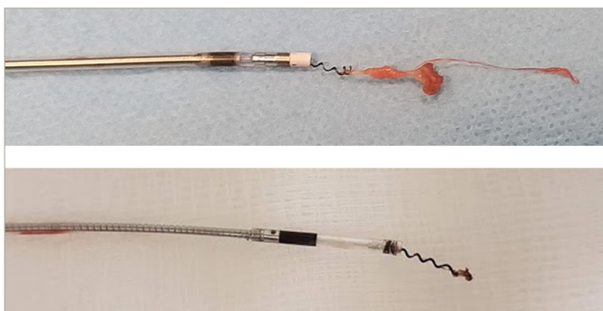
Figure 2: Result of lead entanglement of a stylet-driven lead (top), with screw damage and tissue tearing, and of a lumenless lead (below), with stretching of the screw
